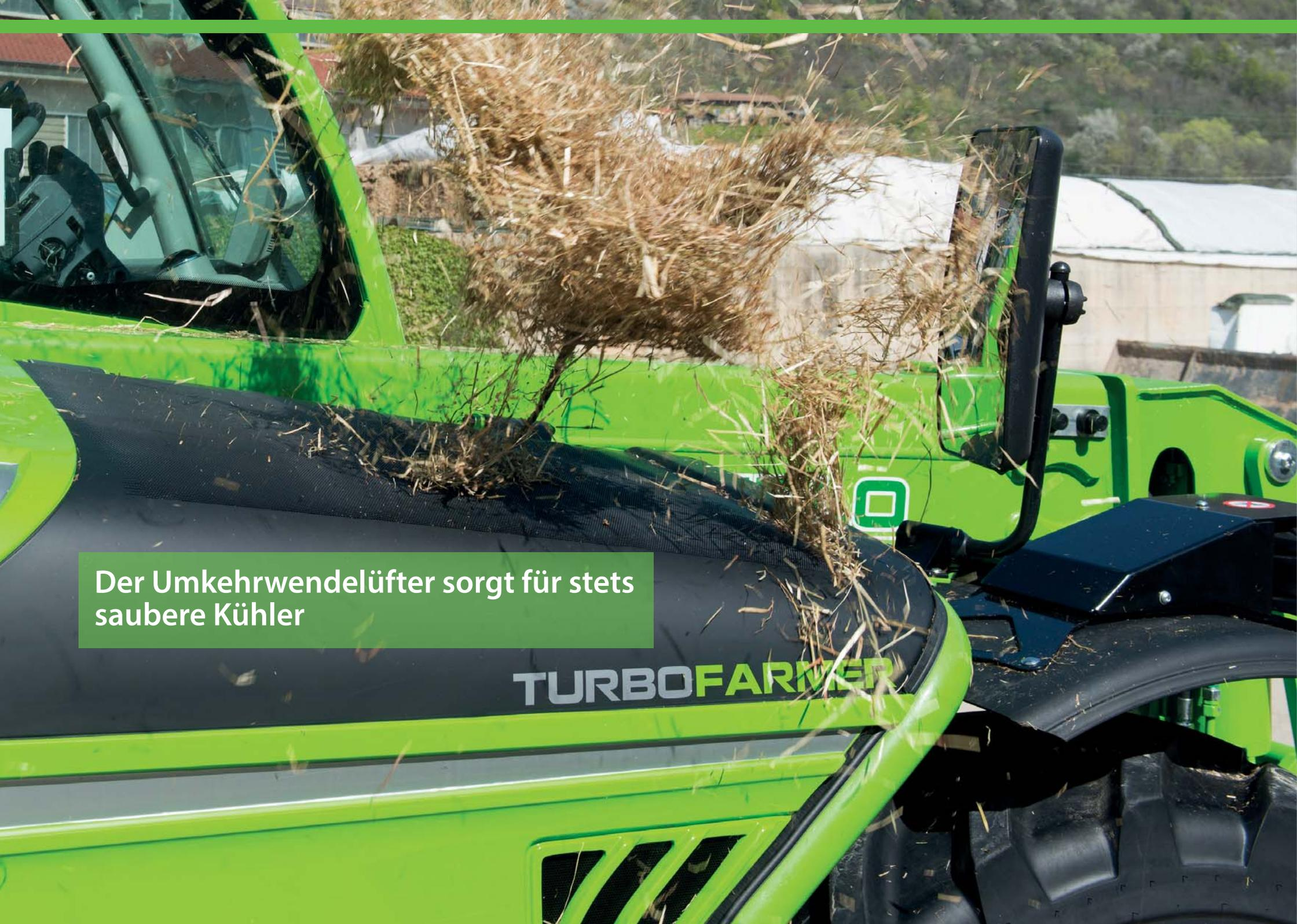
A close-up photograph of a green tractor's engine compartment. A reverse rotating fan is shown in action, blowing a large volume of dry straw and chaff away from the engine area. The tractor's body is painted a vibrant green, and the fan housing is black. The background shows a blurred outdoor setting with a white building and trees.
